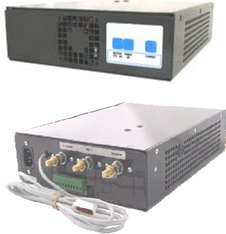
Picture of SR500U , chassis mount with temperature probe option , stud terminals for output
